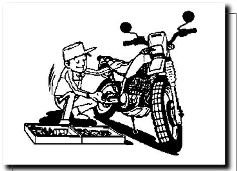
3. On dismantling the motorcycle, always keep paired parts together. This includes gears, cylinders, pistons and other parts submitted to natural wear in pairs. Paired parts must always be reassembled or replaced together.
