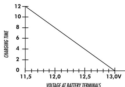
MONITORING GRAPH TO DETERMINE BATTERY CONDITION
