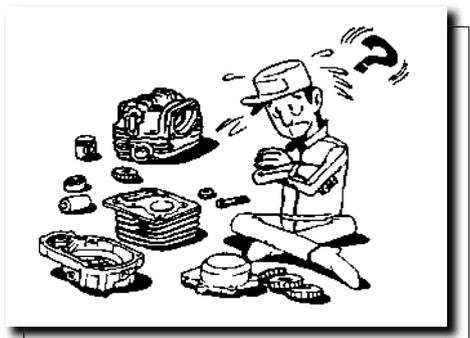
4. While dismantling the motorcycle, clean all the parts and lay them out on trays in the order dismantled. This speeds up reassembly and ensures the correct fitting of all the parts.
