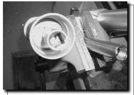
Have ready a suitable sized container in which to drain off the hydraulic fluid from each bar (pump the fork stem assembly in order to ensure it is completely drained).
